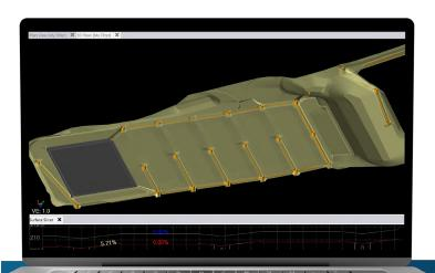
The centerpiece of Severino's construction software buildout is Trimble Business Center (TBC). With a powerful combination of survey and construction functions, TBC helps users manage construction data across an entire project lifecycle—including estimating earthwork and material quantities for bids, preparing data for construction stakeout, building 3D models to optimize machine operation, tracking productivity, and delivering first-class as-built documentation.
