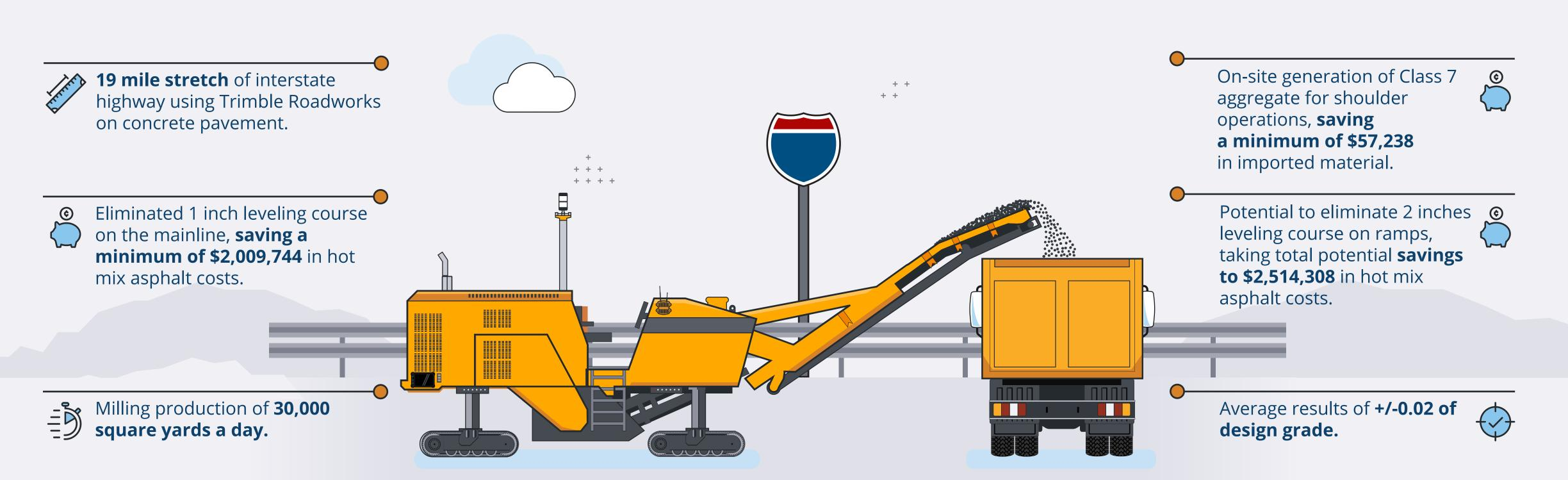
Actual profile milling abstract, submitted by a general contractor to use Trimble® Paving Solutions for Milling Machines on a 19-mile stretch of interstate highway.
