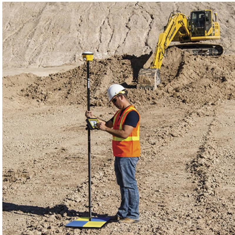
This AeroPoint acted as the sole GCP in the model, and was placed by laying the target on an AeroPoint stencil over a control point known in local coordinates. The drone used five batteries to cover the whole site, and completed the flight in 90 minutes.
