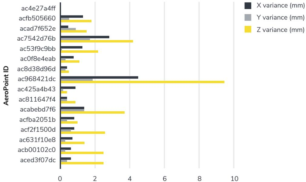
In the second flight, we again calculated AeroPoint positional accuracy. All AeroPoints again reported internally consistent numbers as processed using the known-point method, with no individual point getting less than 1cm accuracy, and most falling well better than that value in the height dimension.
