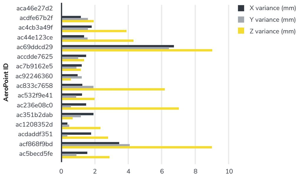
For our first flight, we calculated the variances in each dimension for all the AeroPoints used in this survey. They reported internally consistent numbers as processed using the known-point method. This is where the coordinates of the AeroPoint placed over the known control point are used as the origin to calculate the positions of the remaining AeroPoints.
