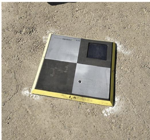
Note that the checkpoints along the left side of the site are actually outside of the drone's flight zone. We wanted to test nonoptimal surveying which is dictated by 107 restriction of flying over non-participants, and this layout makes the checkpoint data used here the worst-case scenario when it comes to placement.
